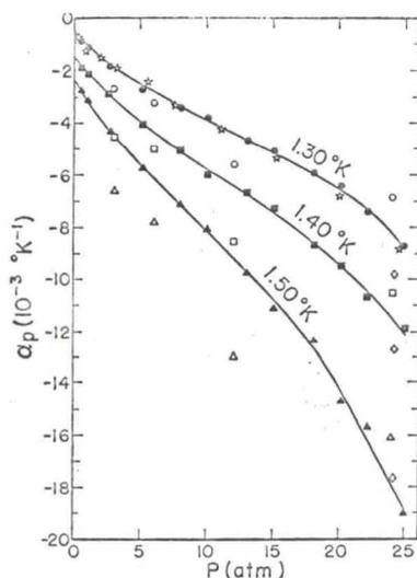
FIG. 4. Thermal expansion coefficient of He<sup>4</sup> along the 1.30, 1.40, and 1.50°K isotherms. The closed symbols are the present results, the corresponding open symbols are the results of Mills and Sydorik (Ref. 15). The diamonds are the results of Grilly and Mills (Ref. 5), given at 24 atm at these same temperatures. The stars are the results of Boghosian and Meyer (Ref. 14) at 1.30°K.
