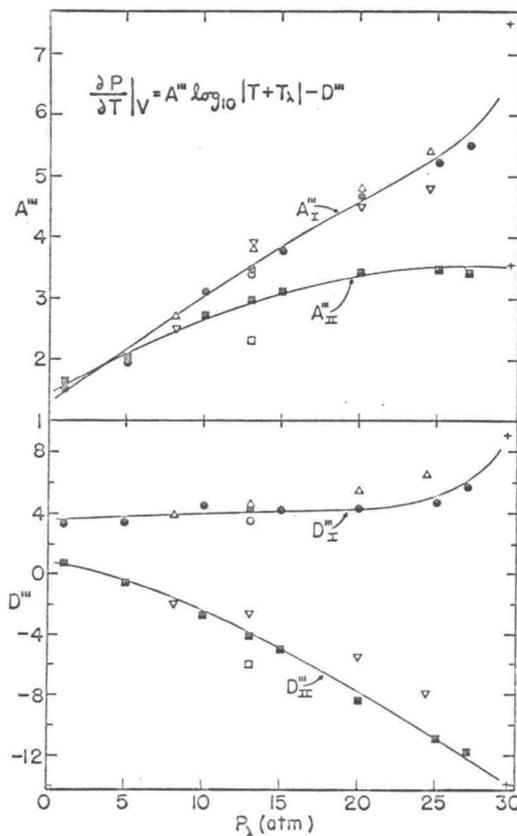
Fig. 9. Parameters  $A'''$  and  $D'''$  (in  $\text{atm deg}^{-1}$ ) for a logarithmic fit to the slope  $(\partial P / \partial T)_\lambda V$ . Black circles and squares: present results. Open triangles: Lounasmaa and Kaunisto (Ref. 23); open circles and squares: Lounasmaa (Ref. 25), + Kierstead (Ref. 24).
