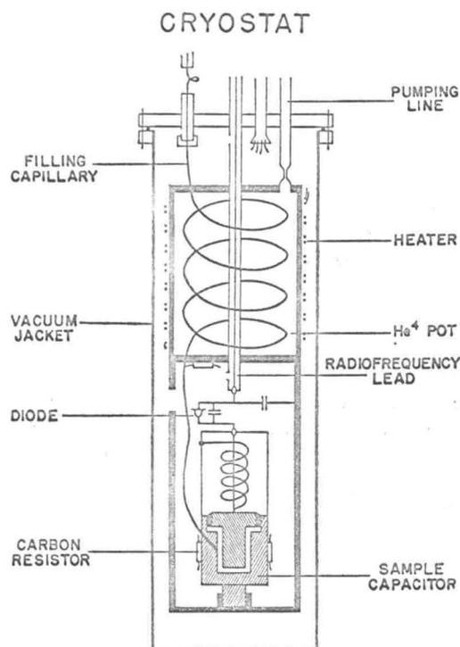
FIG. 1. Schematic diagram of the density cell and He<sup>4</sup> pot for the temperature range between 4.2 and 1.25°K. The vacuum jacket is surrounded by liquid He<sup>4</sup> at 4.2°K.
