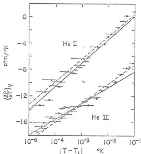
FIG. 10. Comparison of the calculated  $(\partial P/\partial T)_V$  at 13 atm with that measured by Lounasmaa. Solid lines: Logarithmic fit by Lounasmaa. Open circles: experimental points of Lounasmaa (Ref. 25). Closed circles: experimental points of Lounasmaa and Kaunisto (Ref. 23). Dashed lines:  $(\partial P/\partial T)_V$  as calculated from our data by interpolation.
