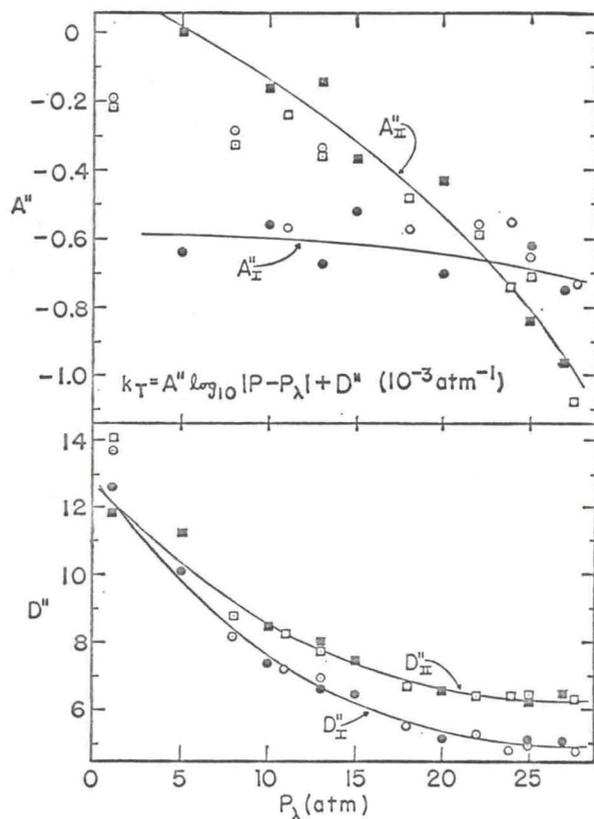
FIG. 11. The parameters  $A''$  and  $D''$  (in  $\text{atm}^{-1}$ ) for the logarithmic fit to  $k_T$ . Circles are for  $T > T_\lambda$ ; squares are for  $T < T_\lambda$ . Black circles and squares: present direct calculations from experiment; circles and squares with dot: cylindrical approximation calculations; open circles and squares: Grilly (Ref. 18).
