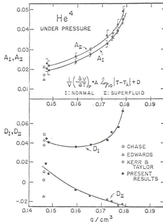
FIG. 7. The parameters  $A$  and  $D$  (in  $\text{deg}^{-1}$ ) of the logarithmic plot for  $\alpha_P$  as a function of density along the transition and comparison with results of other authors at saturated vapor pressure.
